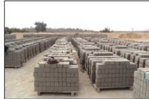
7. Producing building materials from the ashes
